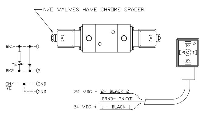
DIN CONNECTOR WITH RECTIFIER-- HTI PART 250-019
